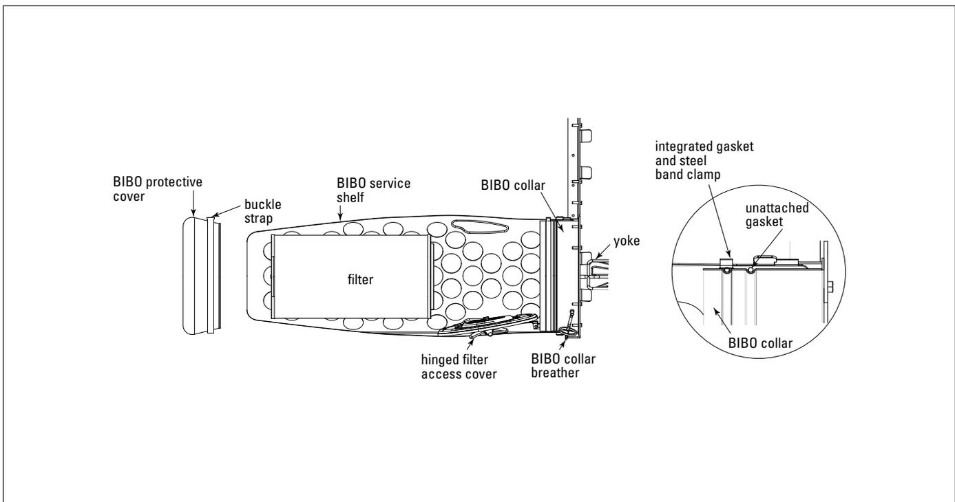
Initial Filter Installation of BIBO
